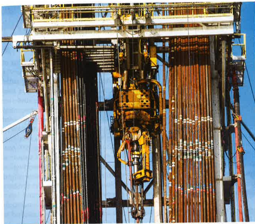
The topdrive (center of the photo) is a defining component of modern drilling systems and enabled a step-change in efficiency when it was introduced. It continues to be critical to automation efforts. Source: Getty Images.
